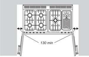
A clearance of 130mm is required if the cooker is near a corner of the kitchen to allow the oven doors to open.
